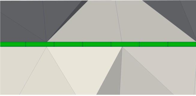
Fig. 22: Cut through the volume elements, to see the nonconforming interface.
