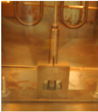
Fig. 10. Magnetic circuit of soft magnetic material placed in the chamber with controlled temperature for the experimental validation
