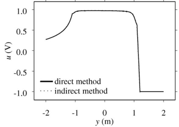
Fig. 3 Potential obtained with the indirect and the direct method in the dielectric and the air gap
