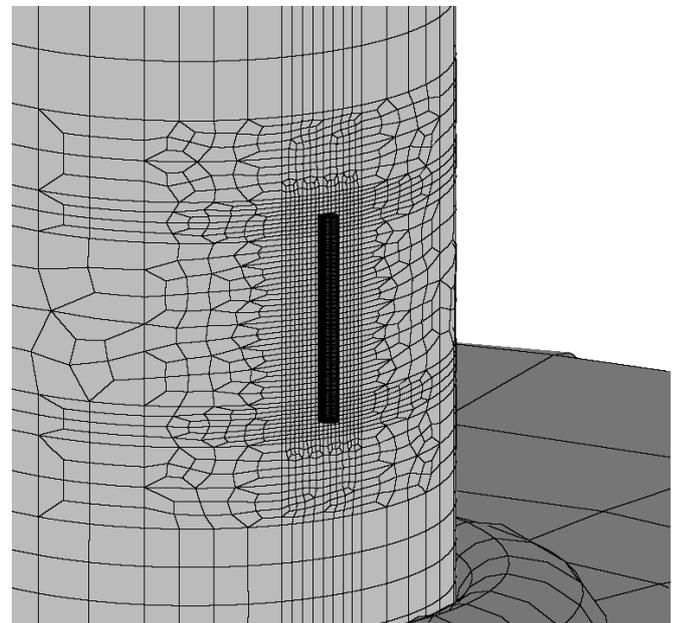
Fig. 6 Detail of Fig. 5, conducting particle on a spacer
