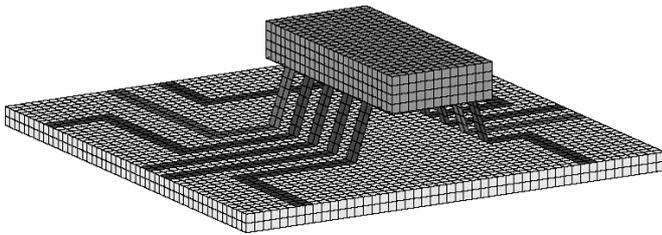
Fig. 4 Chip connected to a printed circuit board
