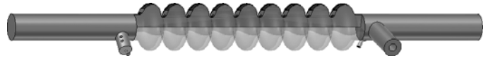
Fig. 12. Geometrical model of the TESLA 3 rd harmonic cavity used to set up a partially symmetric mesh. Initially, in the resonator region, only \frac{1}{4} of the model is used for meshing. In a subsequent step, the obtained tetrahedral elements are mirrored into the missing quadrants. Special care has to be taken in the interface planes.
