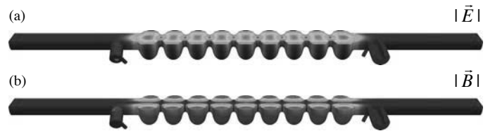
Fig. 13. Distribution of the absolute value of the electric field strength in (a) and the absolute value of the magnetic flux density in (b) for the operating mode. The upper part of the geometry is suppressed for visualization reasons.
