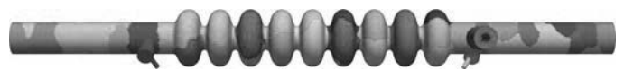
Fig. 8. Partitioning of the computational domain among 64 processes. A unique color is assigned to each of the sub domains. Their quantity can be adjusted according to the problem size and available computational resources.
