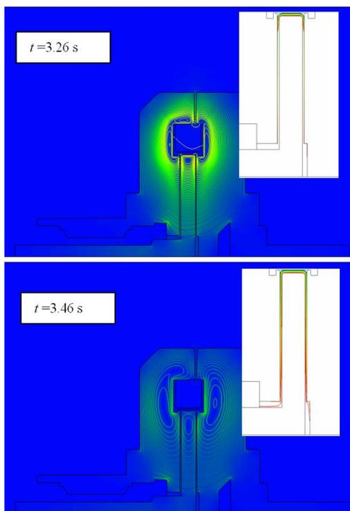
Fig. 21. Magnetic flux lines distributions and fluid velocity distributions for chosen time instants in disk shape MR clutch after switching off the supply voltage
