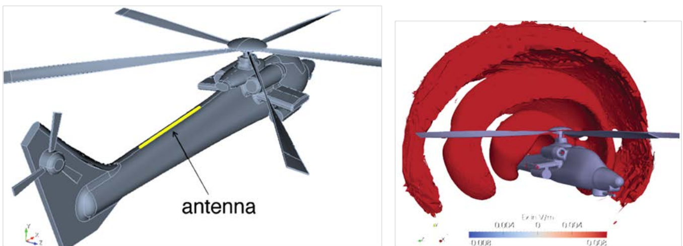
Figure 6: Field-cable coupled DGFEM simulation of a helicopter antenna (left) and the radiated electric field intensity [16]
