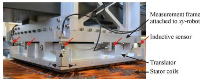
Fig. 30. Photo of the realized planar actuator and part of the measurement setup.
