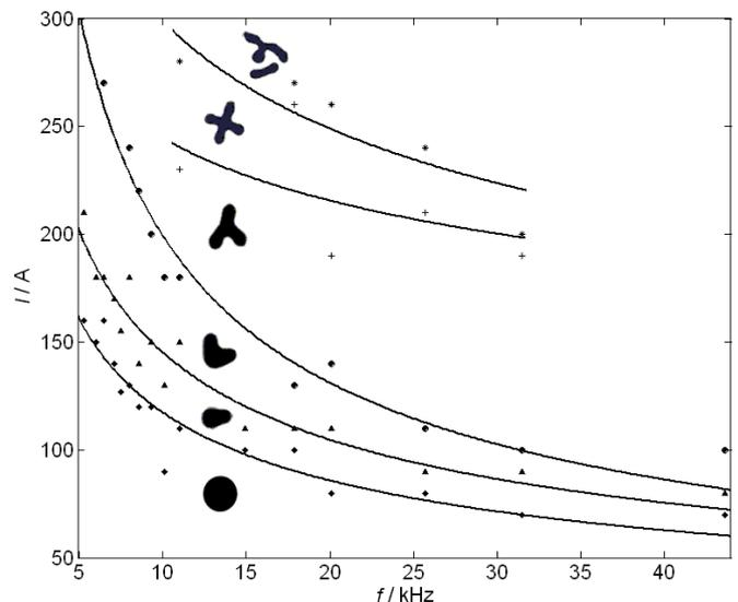
Fig. 16. Phase diagram of the inductor current vs. frequency for a liquid metal sheet (Galinstan), with thickness of 3mm.
