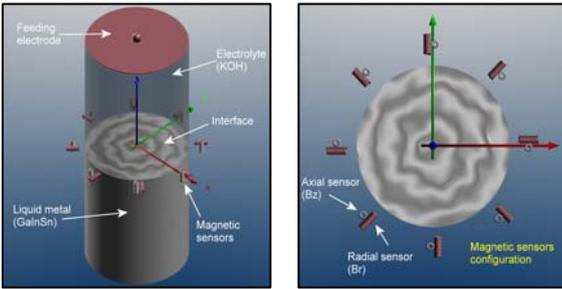
Fig. 22. Cylindrical two-fluid-cell as highly simplified model of an aluminium reduction cell with eight 2D fluxgate sensors (Fluxset<sup>®</sup> FXM-205) positioned on a circular ring near the cylinder wall
