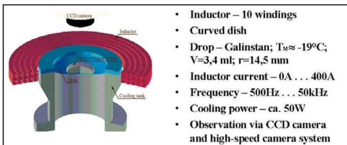
Fig. 13. Experimental setup for studies of the “drop”
