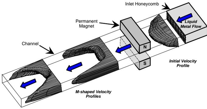
Fig. 4. Velocity distribution at the flow around the magnetic obstacle obtained by simulation [6]
