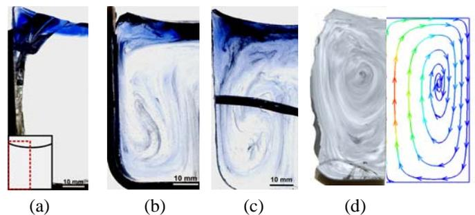
Fig. 20. Cuts through the solidified glass probes, (a) – after 5 min indirect heating, (b) – after 5 min direct heating, (c) – after 5 min with Lorentz force upwards, (d) - after 25 min with Lorentz force upwards, and simulated velocity profile
