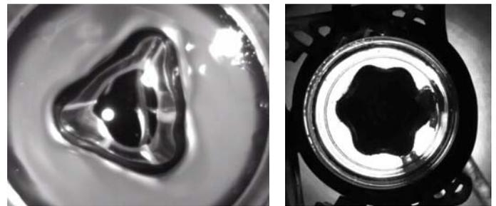
Fig. 15. Shape deformations of liquid metal drops in alternating magnetic field
