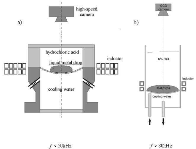
Fig. 14. Setup for experiment with metallic drops, with modification of parameters: critical current  $I_C$ , frequency  $f$ , drop volume  $V$ .
