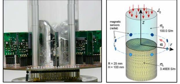
Fig. 23. Experimental setup of the cylindrical two-fluid-cell with the magnetic sensor ring (left) and the numerical model used for simulations (low-conducting electrolyte KOH,  $\sigma_2 = 100.0$  S/m, high-conducting liquid metal Galinstan,  $\sigma_1 = 3.48E6$  S/m, right)
