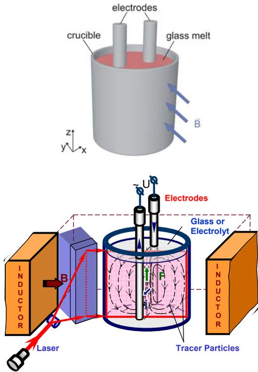
Fig. 17. Experimental setup for electromagnetic stirring of glass melts
