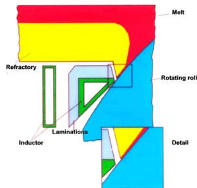
Fig. 9. Continuous steel casting and stopping the melt flow in the gap by means of electromagnetic fields
