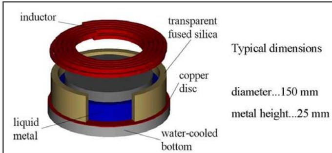
Fig. 12. Experimental setup for studies of the “annular gap”
