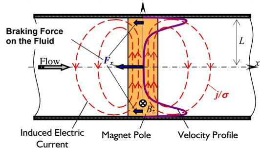
Fig. 3. Braking force caused by the permanent magnet acting on the fluid
