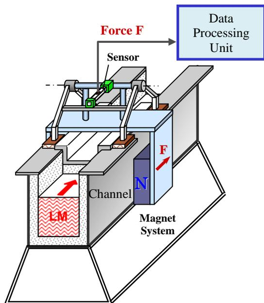
Fig. 8. Scheme of an industrial prototype of a Lorentz force anemometer applied to liquid metal (LM) flowing in a channel
