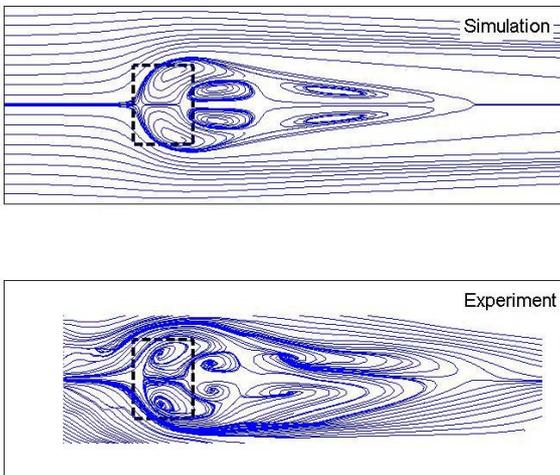
Fig. 6. Comparison of numerical simulation and experiment of the fluid flow around a magnetic obstacles
