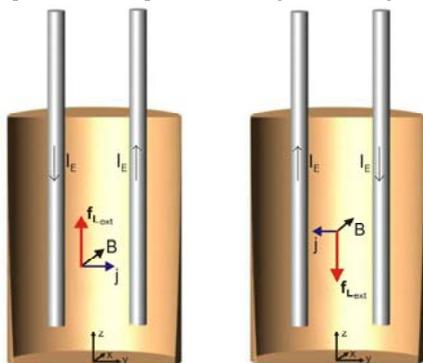
Fig. 18. Lorentz forces  $f_L$  impressed to the glass melts in opposite directions
