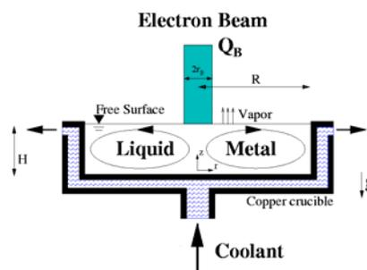
Fig. 10. Crucible free evaporation of liquid metal
