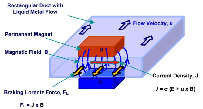
Fig. 2. Basic principle of "magnetic obstacle" acting on conducting fluid flow
