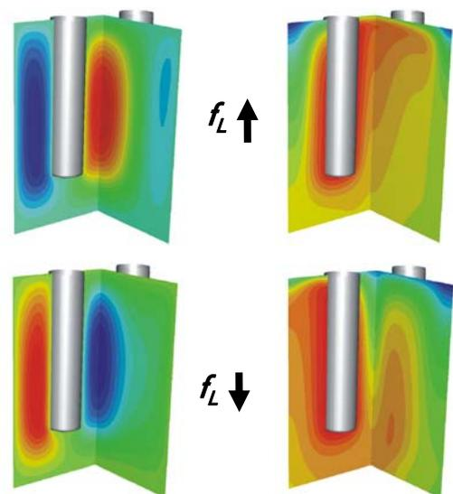
Fig. 21. 3D simulation of the flow rate distribution (velocity, left) and temperature profiles (right) for different directions of the Lorentz forces
