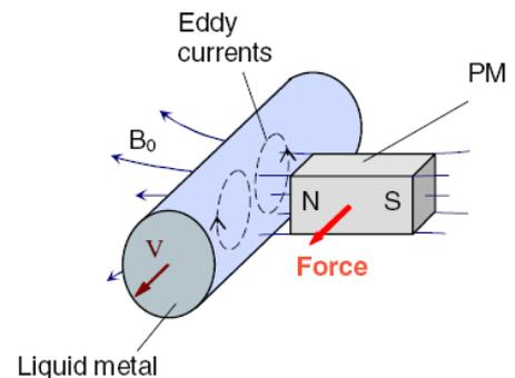
Fig. 7. Principle sketch of the Lorentz force velocimetry showing the action of a permanent magnet (PM) upon the flow of an electrically conducting fluid.
