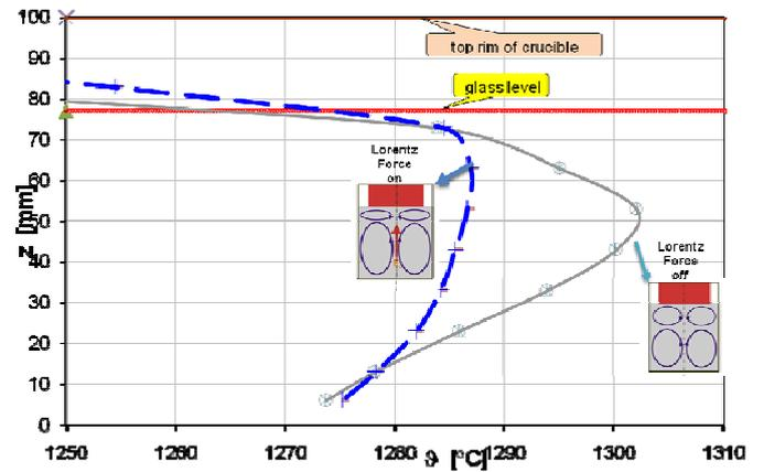
Fig. 19. Vertical temperature profiles, without magnetic field (small circles) and after turning on the external Lorentz forces (small triangles)
