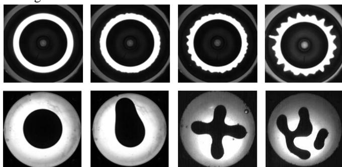
Fig. 11. Pinch instability in a liquid metal sheet: temporal development of the free surface, for „Annular Gap“ (upper row) and „Drop“ (lower row).
