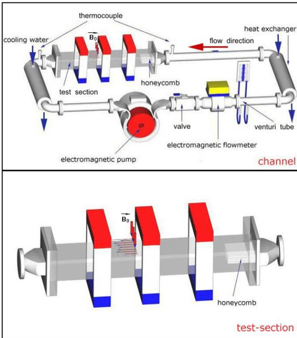
Fig 1. Experimental liquid metal loop (top), test section (bottom)
