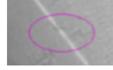
Fig. 1. Transmission electron microscopic image of a domain wall pinned to a dislocation. The domain wall is pinned in the middle of the dislocation line.
