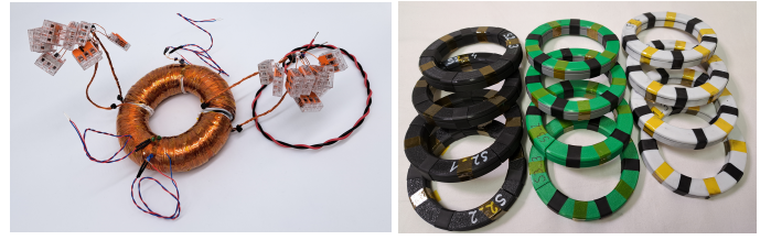
Fig. 3. Open ring measurement system for characterizing SMM powders featuring low material densities on the left side, and the 12 slotted sample containers filled with three different iron powders on the right side.
