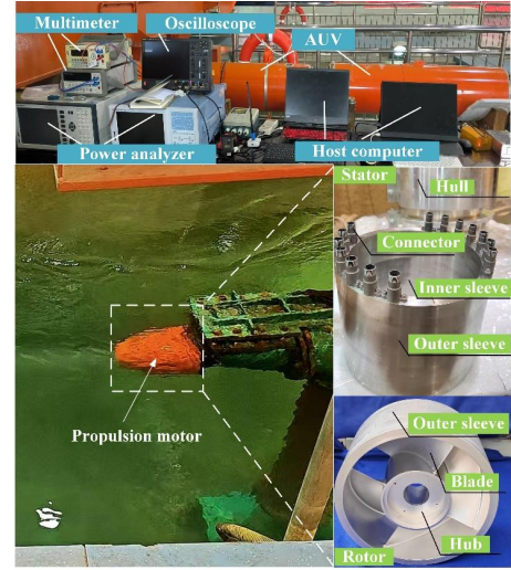
Fig. 7. Test platform and main parts of shaftless propulsion motor
