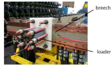
Fig. 4. Induction loader mounted to the railgun breech.
