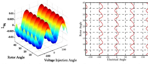
Fig. 1. Variation of the inductance according to the rotor position and current
