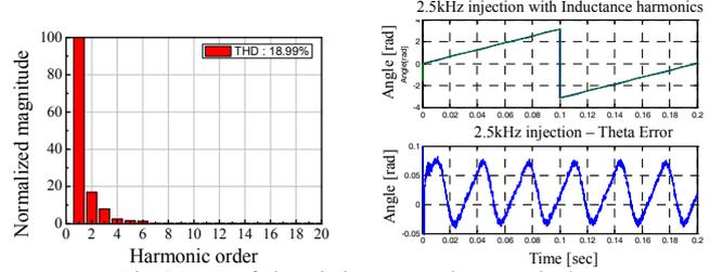
Fig. 2. THD of phase inductance and current ripple
