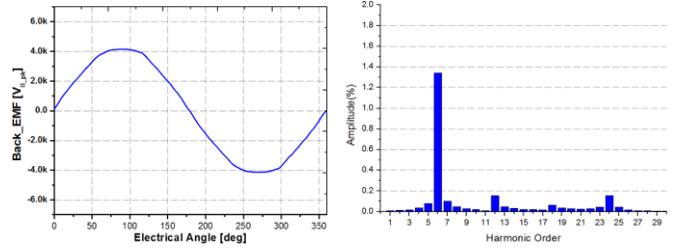
Fig 7. The Torque ripple and back EMF at the rated condition
