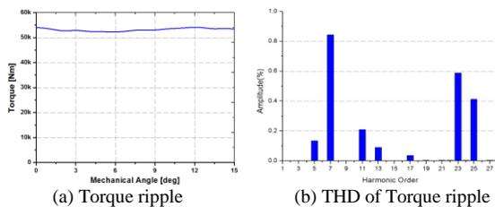
Fig 6. The Torque ripple and THD at the rated condition
