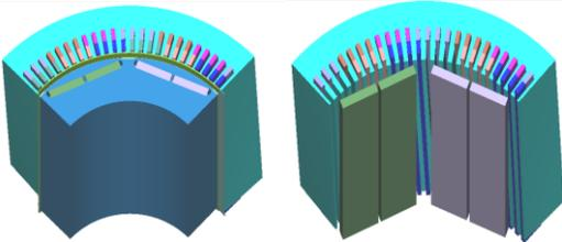
Fig. 4. The structure of IPMSG
