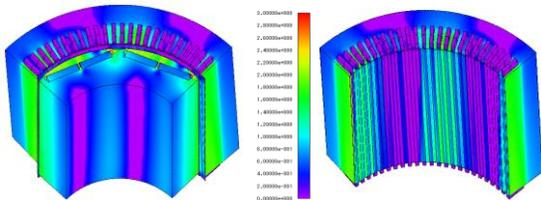
Fig 5. The flux density distribution of designed IPMSG at the rated condition (5.6MW, 1096rpm)
