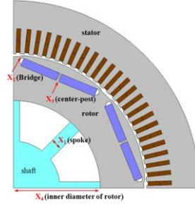
Fig. 1 The design variable of IPMSG taking account of mechanical analysis
