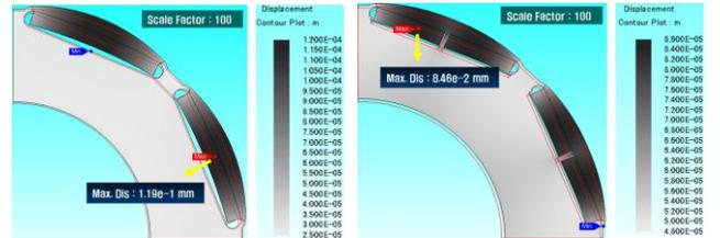
Fig. 3. Comparison results of mechanical displacement analysis
