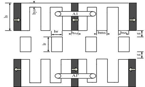
Fig. 1. Two-dimensional topology of E-core AFFSPM machine
