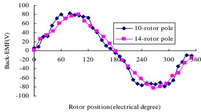
Fig. 4. Back-EMF waveforms of the two E-core machines at 750r/min
