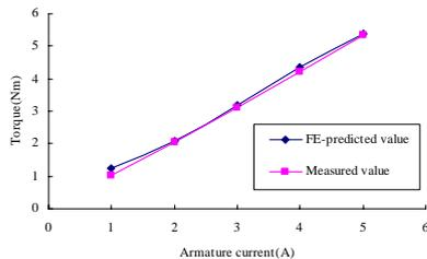
Fig. 5. Torque-current characteristics of the 6/14-pole E-core machine
