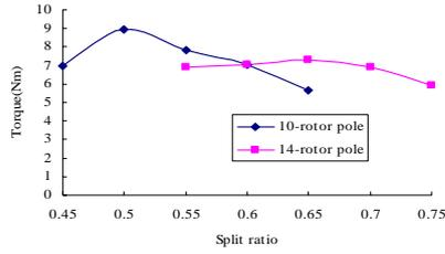
Fig. 3. Variation of torque with split ratio
