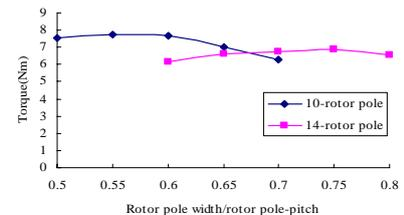
Fig. 2. Variation of torque with ratio of rotor pole width to rotor pole-pitch
