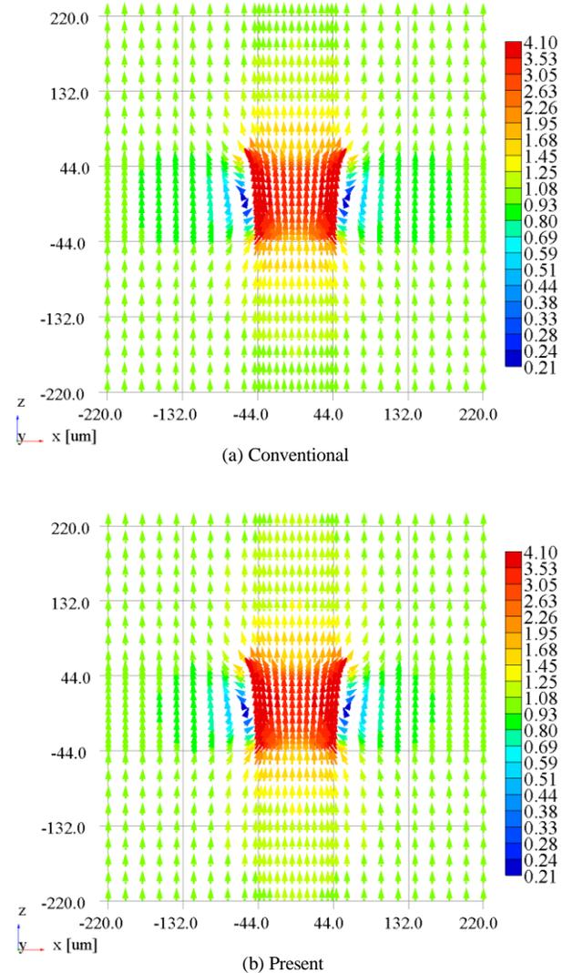
Fig. 4. Distribution of magnetic flux density on  $x$ - $z$  plane for model 2
