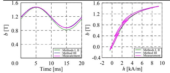
Fig. 2. Numerical results obtained from Methods I – III (minor loops).
