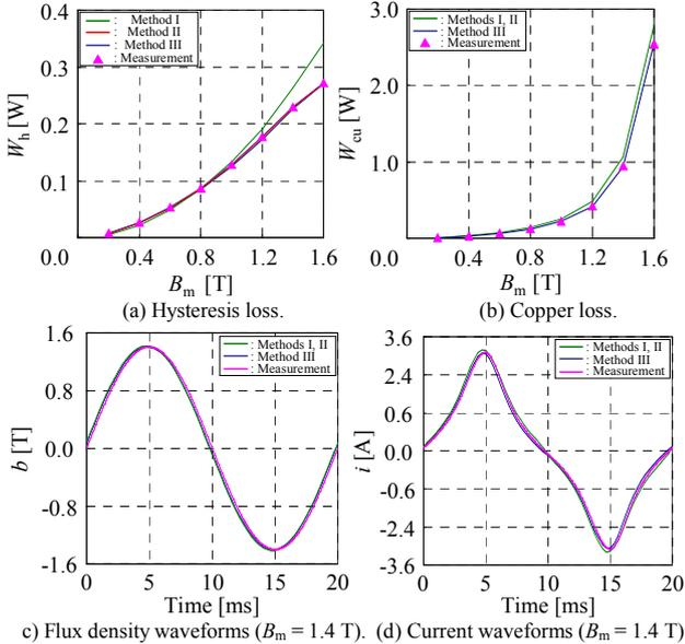
Fig. 1. Numerical results obtained from Methods I – III (symmetric hysteresis loops).
