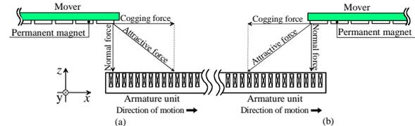
Fig. 2. Forces exerted in the mover at the end edge: (a) entry interval (entrance end) and (b) ejection interval (exit end)
