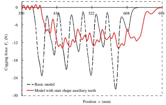
Fig. 6. Waveform of end edge's cogging force of each model.
