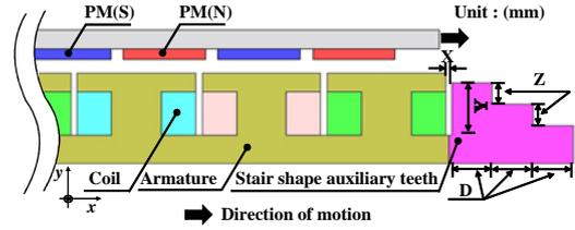
Fig. 5. Proposed model with auxiliary teeth of stair shape.
