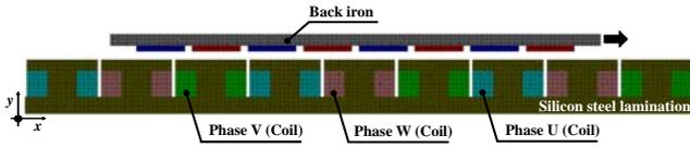
Fig. 3. Element divisions of the basic model for 2-D numerical analysis.
