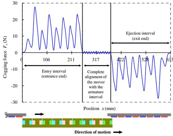
Fig. 4. Cogging force waveform of basic model.
