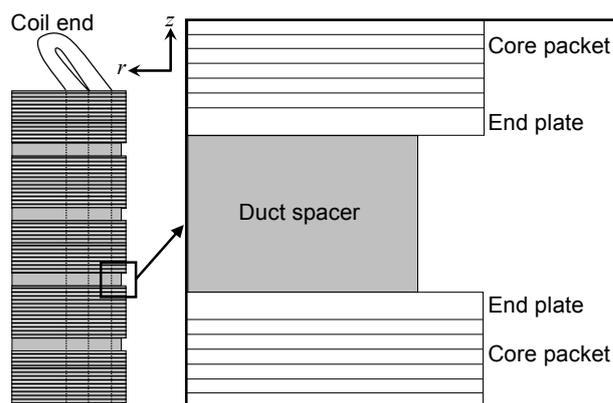
Fig. 1. Outline of stator core.
