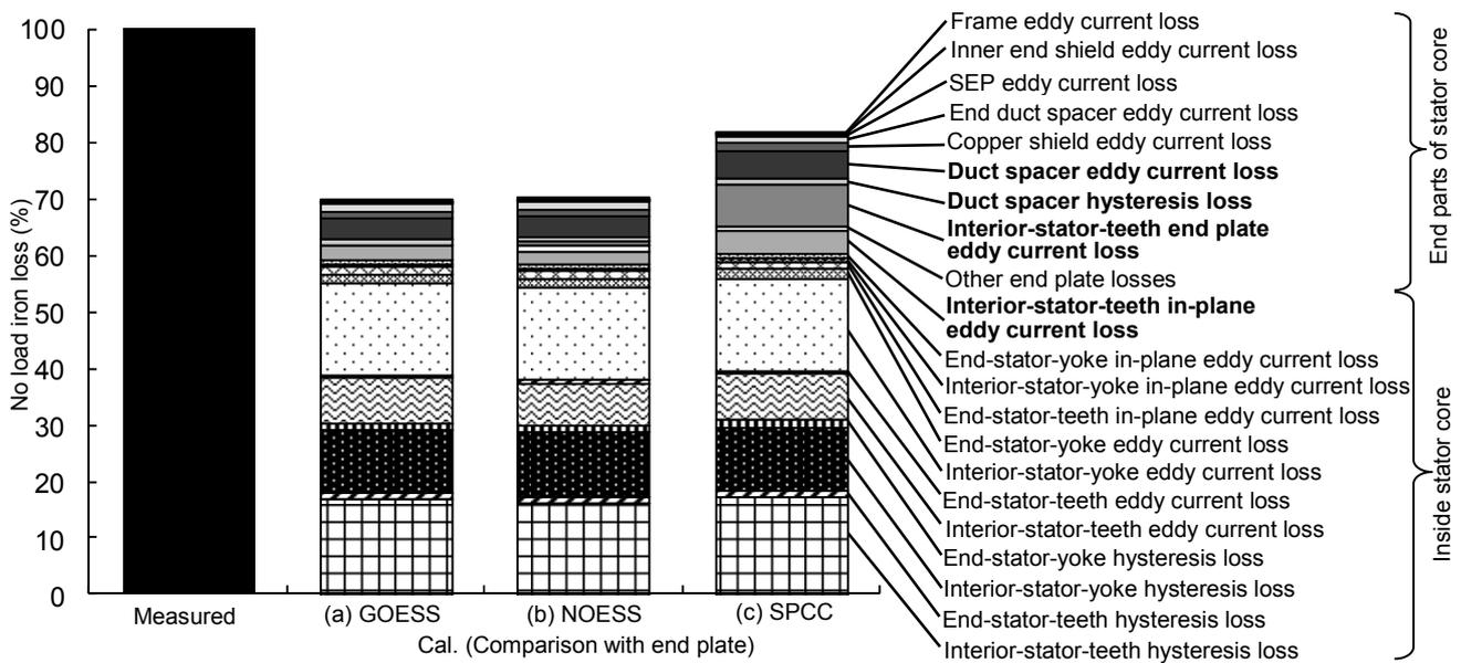
Fig. 4. Experimental and calculated no-load iron losses.
