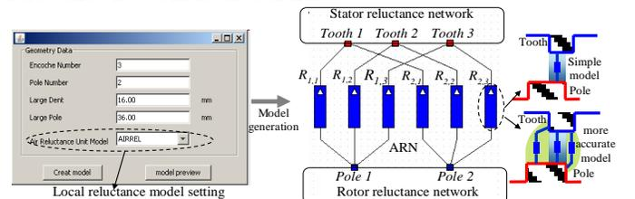
Fig. 2. Implimented tool for automatic generation and setting of ARN.
