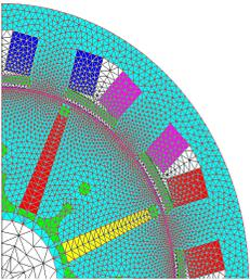
Fig. 4. 1/4 Mesh of the 12/8 PMSM
