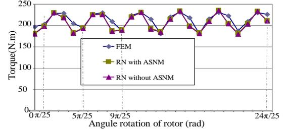
Fig. 6. Torque of the machine calculated by three methods
