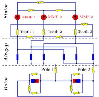
Fig. 5. 1/4 Reluctance network of the 12/8 PMSM
