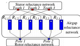
Fig. 1. Complete RN of three teeth and two poles machine an electrical period. Thus, harmonics values of the torque and the back-emf will be available.
