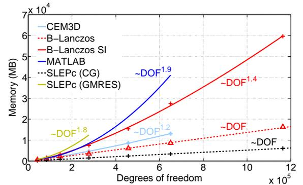
Figure 3: Memory consumption for a billiard cavity. Different number of curvilinear tetrahedrons is used within the solvers.
