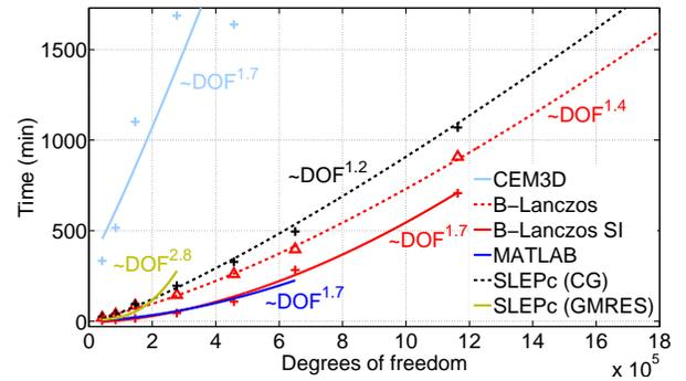
Figure 2: Time consumption for a billiard cavity. Different number of curvilinear tetrahedrons is used within the solvers.
