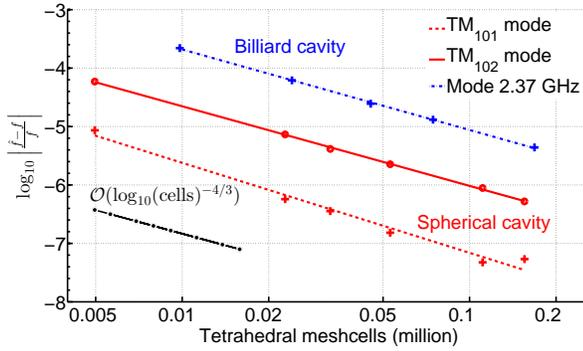
Figure 1: Relative deviation of the numerically obtained values of  $\hat{f}$  to the reference results  $f$  as a function of the degrees of freedom for a spherical and billiard resonator. The first two worst computed degenerated mode eigenfrequencies are considered for the spherical cavity, whereas for the billiard cavity the 2.37 GHz mode eigenfrequency is determined.
