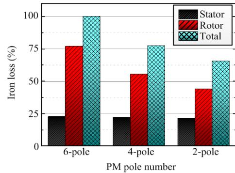
Fig. 8. Comparison of iron losses at various pole-changing operations.
