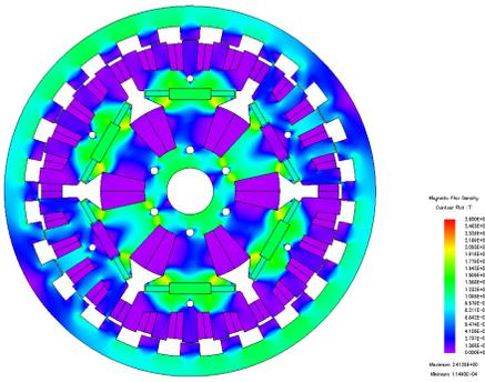
Fig. 4. Magnetic flux density distribution at 2-pole operation.
