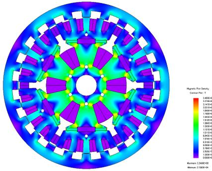
Fig. 2. Magnetic flux density distribution at 6-pole operation.
