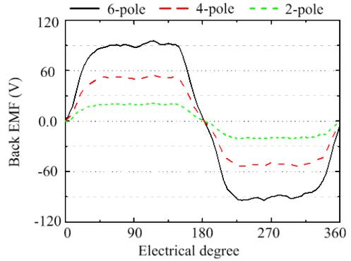
Fig. 6. Back EMF waveforms at various pole-changing operations.
