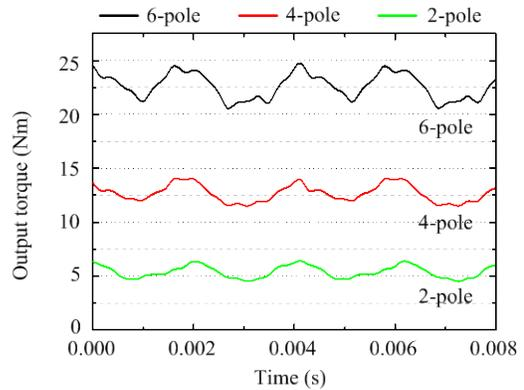
Fig. 7. Output torque waveforms at various pole-changing operations.
