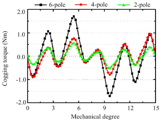
Fig. 5. Cogging torque waveforms at various pole-changing operations.
