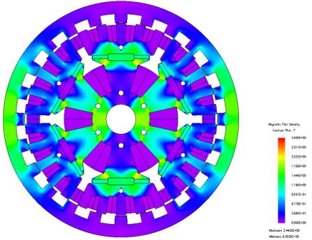
Fig. 3. Magnetic flux density distribution at 4-pole operation.
