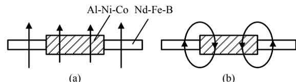
Fig. 1. Magnet arrangement for each PM pole. (a) PM materials in same flux direction. (b) PM materials with opposite flux direction.
