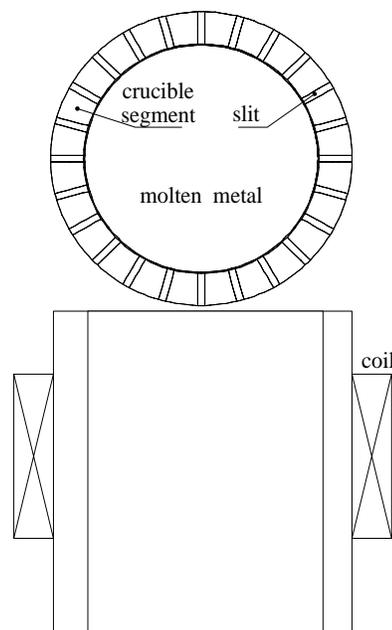
Fig. 1. Schematic diagram of a cold crucible and the rotational symmetry
