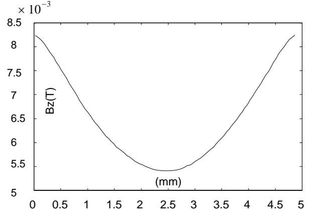
Fig. 3. The distribution of the computed magnetic flux density on the surface of the molten metal along the circumferential directions in the center position of the coil energized with harmonic current at 20 kHz
