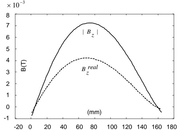
Fig. 4. The distribution of the computed magnetic flux density at points of the slit center which are on the surface of the molten metal along the z-coordinate direction with harmonic current of 20 kHz
