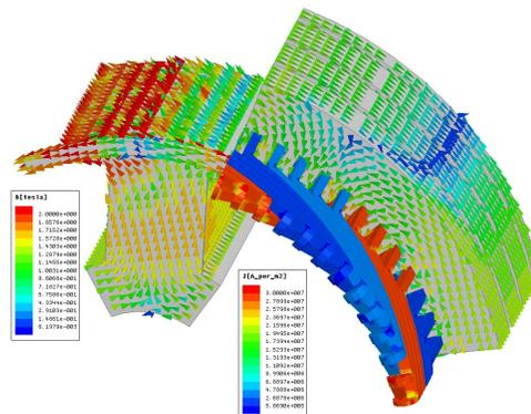
Fig. 2. Plot of flux density, induced eddy currents and source currents
