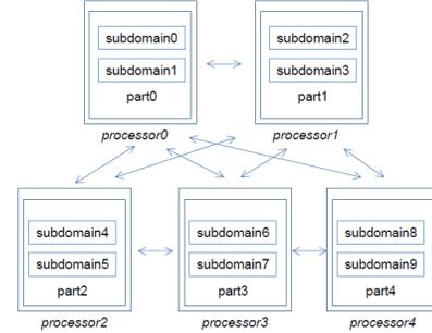
(b) Data distribution and communication in the parallel processor mode
