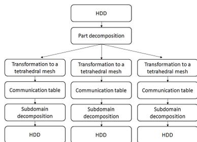
Fig. 3. Procedure for generation of the HDD mesh
