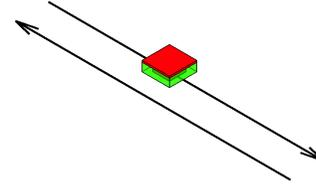
Fig. 2: Power line embedded in the road (arrows) and pick up coil (core in red, coil in green).
