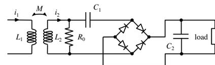
Fig. 3: Circuit model of the inductive power system.
