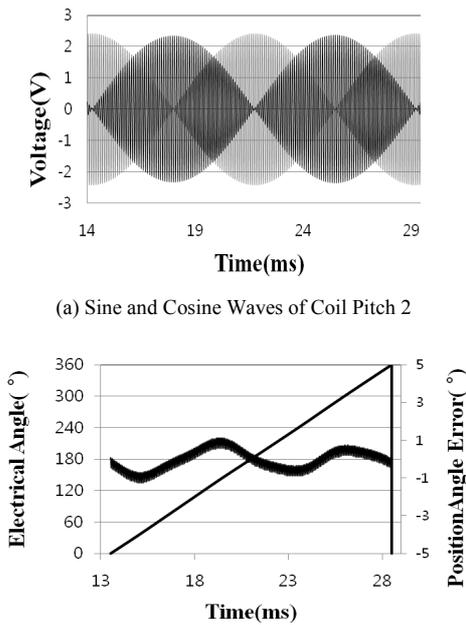
(a) Sine and Cosine Waves of Coil Pitch 2
