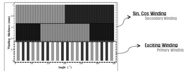
Fig.2. Scheme of Slotless VR Resolver Winding
