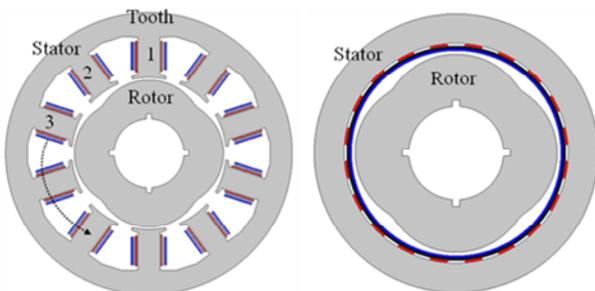
Fig. 1. VR Resolver of slot type and slotless type
