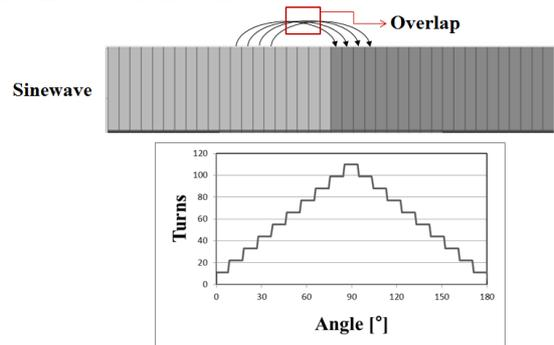
Fig.3. Sine Winding
