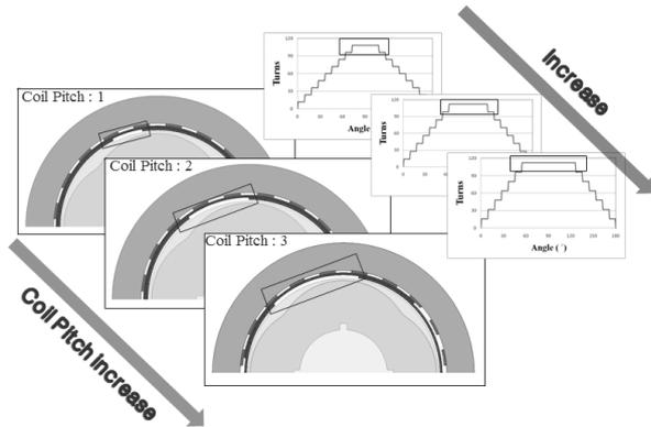
Fig.5. Increase of Coil Pitch
