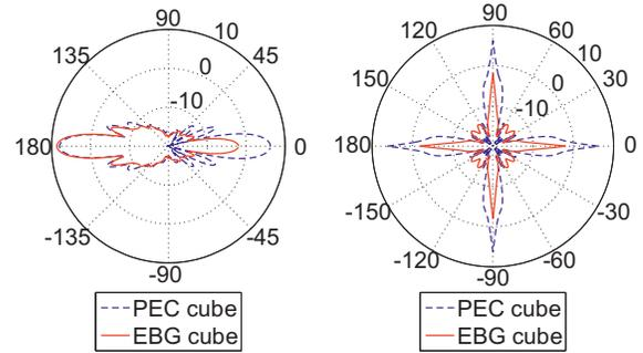
Figure 4: RCS graph in the cases of unshielded and shielded metallic cube at 7.756 GHz. Firstly (left), the plane wave impinges normally at the cube ( $\theta = 0$ ) and the RCS is estimated on E-plane. Secondly (right), the angle of incident plane varies and the RCS value at  $(0, \theta, 0)$  point is plotted.
