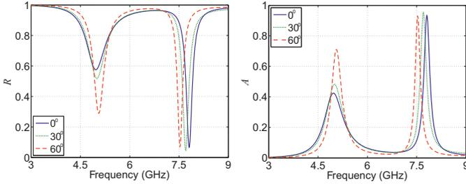
Figure 2: The reflectance  $R$  (left), and absorption  $A$  (right) for the cross-EBG.
