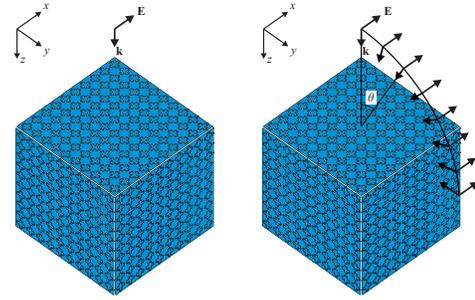
Figure 3: The shielded metallic cube geometry by cross-EBG for the simulation of RCS, when  $\theta$  is fixed (left) and when varies (right).
