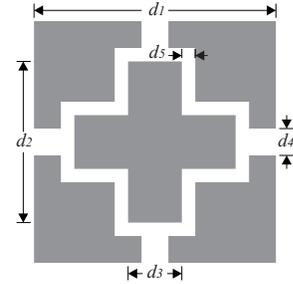
Figure 1: The unit cell of the cross-EBG structure, where  $d_2 = 10$  mm,  $d_3 = 2.5$  mm,  $d_4 = 0.5$  mm and  $d_5 = 1$  mm.
