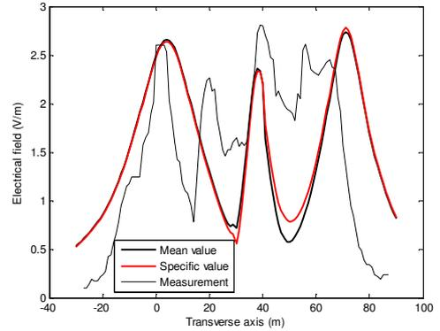
Fig. 4. Radiated electrical field – Simulation and Measurement
