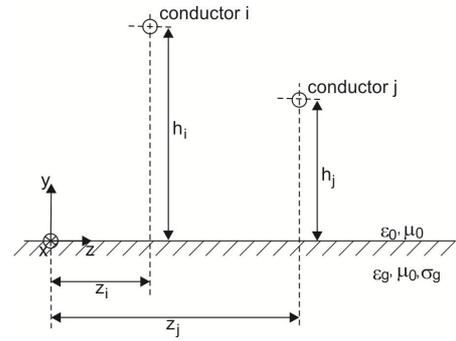
Fig. 1. General configuration of a transmission line
