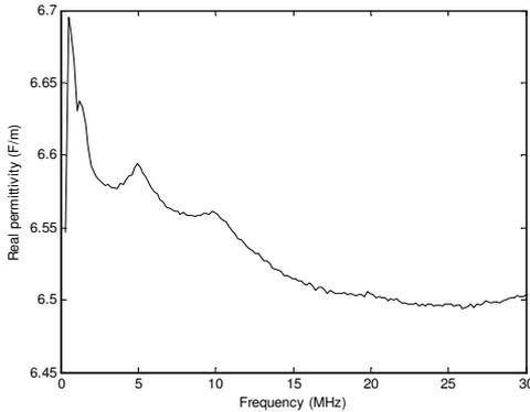
Fig. 2. Real permittivity for the ground sample in the PLC spectrum
