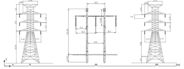
Fig. 3. Sketch of the supports of the transmission line corridor
