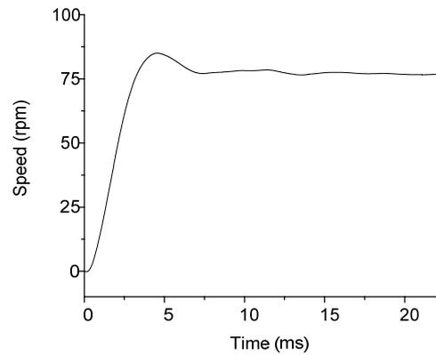
Fig. 3. The speed waveforms during starting.
