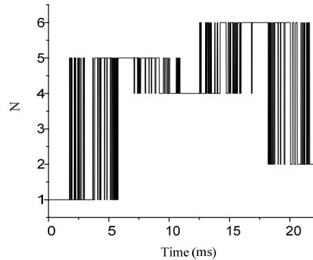
Fig. 4. The sector transition for SVPWM during starting.
