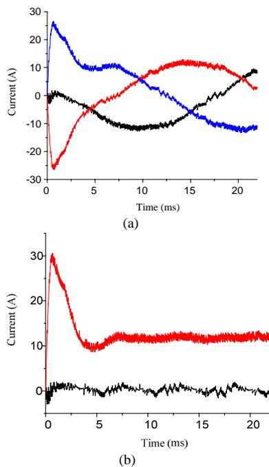
Fig. 2. The starting current waveforms. (a) Three phase current waveforms. (b)  $I_d$  and  $I_q$  waveforms.
