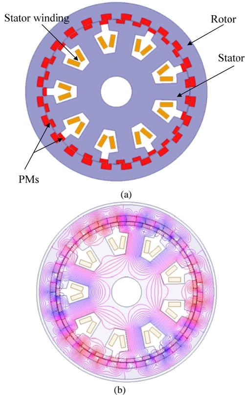
Fig. 1. Dual PM Vernier machine. (a) Structure. (b) Flux distribution.
