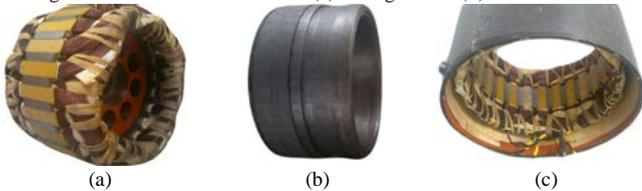
Fig.5. The DSSA VPM prototype (a) inner stator (b) rotor (c) outer stator PM machines, and Torque per unit of Rotor Volume (TRV) of all these VPM machines is larger than  $53 \text{ kNm/m}^3$  compare to a typical value of  $14\text{-}42 \text{ kNm/m}^3$  [5] for a totally-enclosed motors.
