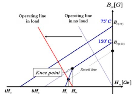
Fig. 2. Characteristic curve of permanent magnet
