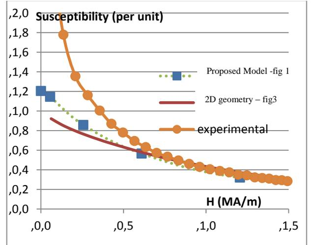
Fig. 4: Comparison of the susceptibility obtained by the proposed method, FEM simulation and experimental tests.
