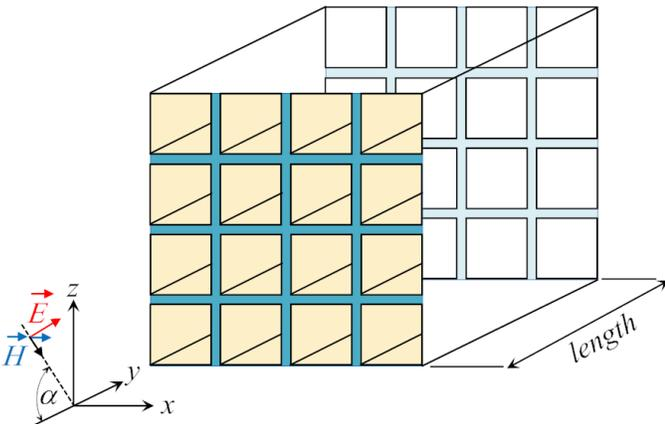
Fig. 1. Basic arrangement, impinging plane wave indicated at an incident angle  $\alpha$ , variable thickness.
