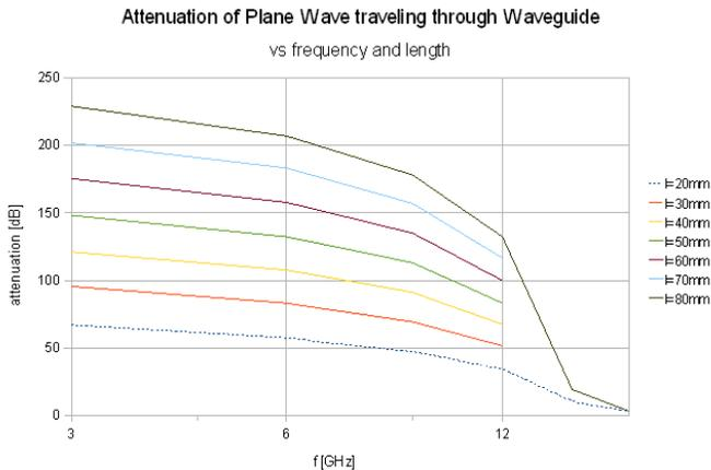
Fig. 3. Attenuation factor at distinct lengths and frequencies.
