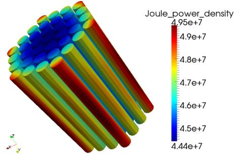
Figure 1: Joule power density for a 4-layers cable with straight wires (C1) (Post-processing realized with Paraview®). [8]
