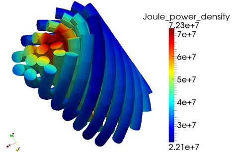
Figure 2: Joule power density for a 4-layers cable with helical arrangement (C2).
