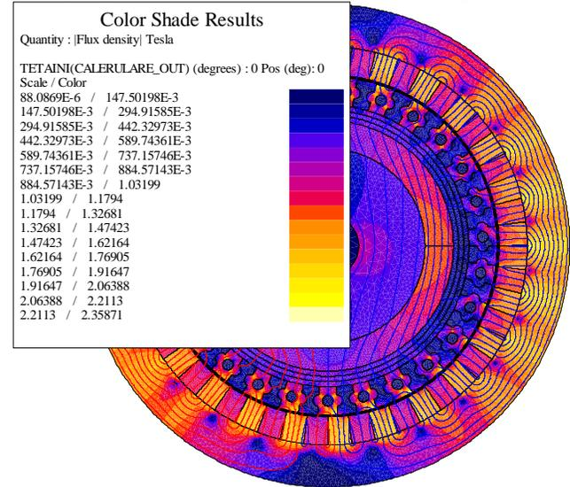
Fig. 1. Flux density & field lines in the active parts of the studied MG.
