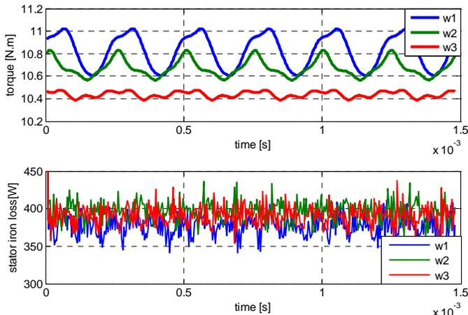
Fig. 2. Torque and iron loss curves for the studied HS-PMSM at rated operating conditions.
