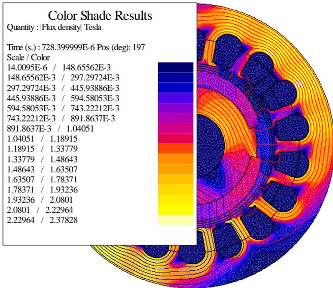
Fig. 1. Flux density & field lines in the active parts of the HS-PMSM.
