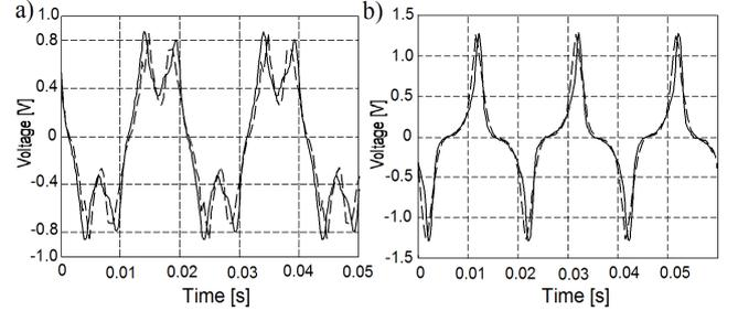
Fig. 4. Voltages of the measurement coil in the rolling direction: a) rotational magnetization, b) alternating magnetization; continuous line – measured waveform, dashed line – calculated waveform.
