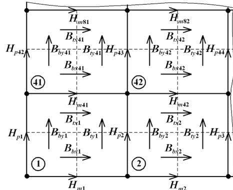
Fig. 2. An example of the description of the field intensity and flux density components
