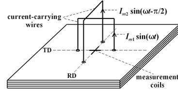
Fig. 3. Measurement system; RD, TD – rolling, transverse direction respectively
