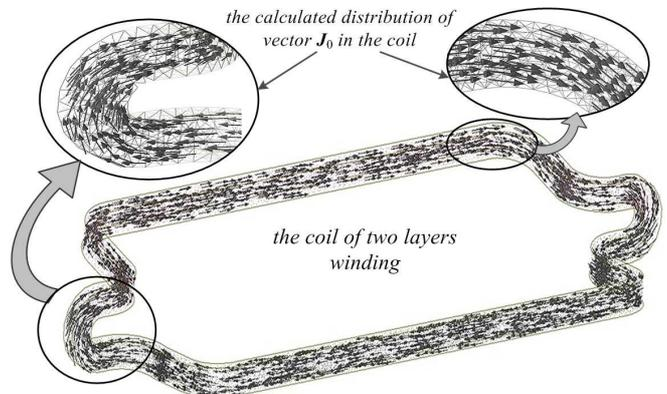
Fig.2. Distribution of current density vector  $\mathbf{J}_0$  in coil of the double layer winding
