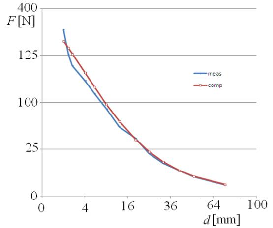
Fig. 4. Force in vertical direction as a function of gap of a pair of magnets length x width x height: 50 mm x 20 mm x 10 mm, magnetized along width
