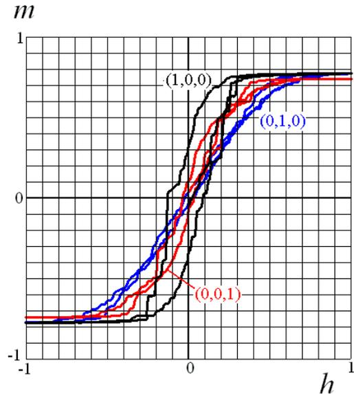
Fig. 1. Magnetizing characteristics of virtually extended rod-shaped dipole cluster of simple cubic structure, with 25% of the dipoles removed from random locations.
