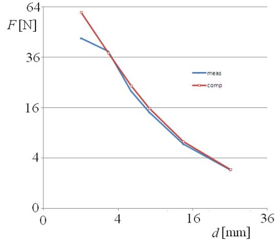
Fig. 5. Force in vertical direction as a function of gap of a pair of magnets length x width x height: 10 mm x 20 mm x 50 mm, magnetized along length
