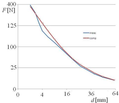
Fig. 3. Force in vertical direction as a function of gap of a pair of magnets length x width x height: 50 mm x 20 mm x 20 mm, magnetized along height
