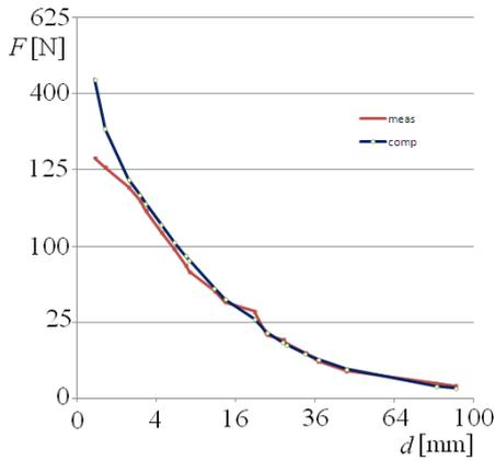
Fig. 2. Force in vertical direction as a function of gap of a pair of magnets length x width x height: 50 mm x 20 mm x 10 mm, magnetized along height
