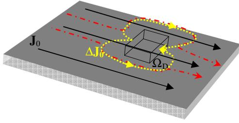
Fig. 1. Sketch of conducting domain  $\Omega$  and of the hole region  $\Omega_D$
