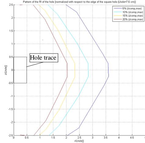
Fig. 2. Contour lines of the normalized norm (with respect to  $|\mathbf{J}_c|$ ) of the current density generated by the compensation source
