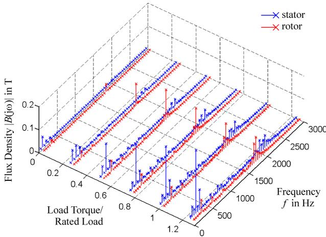
Fig. 2. Load dependent frequency spectrum of the tangential component of the flux density observed in a stator and rotor tooth tip. The fundamental frequency component is not shown, the rotor frequencies are given in a moving rotor coordinate system.
