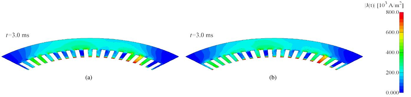
Fig. 1. Current density distribution in a stator sheet at a specific time instant and rated load computed by the harmonic superposition principle (a) and a transient analysis (b).
