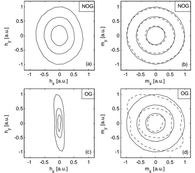
Fig. 3 - Comparison between measured (solid line) and computed (dotted line). The measured magnetic field is used as input for the hysteresis model.
