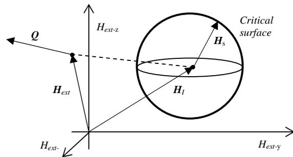
Fig. 1 - Working principle of the vector model.
