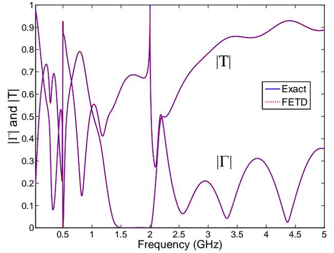
Figure 1: Numerical solution of the reflection ( $\Gamma$ ) and transmission ( $T$ ) coefficients along with the exact solution.
