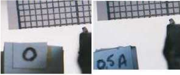
Fig. 14. 0.5 A direct current is set in the coil and a displacement of 0.3 mm is measured as gauge is graduated with 1 mm square.
