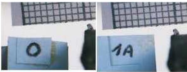
Fig. 15. 1.0 A direct current is set in the coil and a displacement of 0.8 mm is measured as gauge is graduated with 1 mm square..
