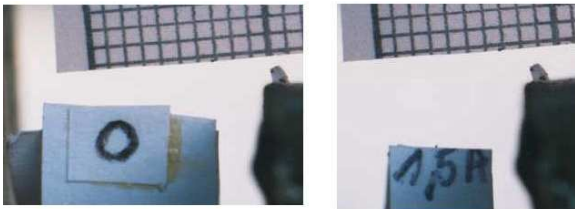
Fig. 16. 1.5 A direct current is set in the coil and a displacement of 1.7 mm is measured as gauge is graduated with 1 mm square..
