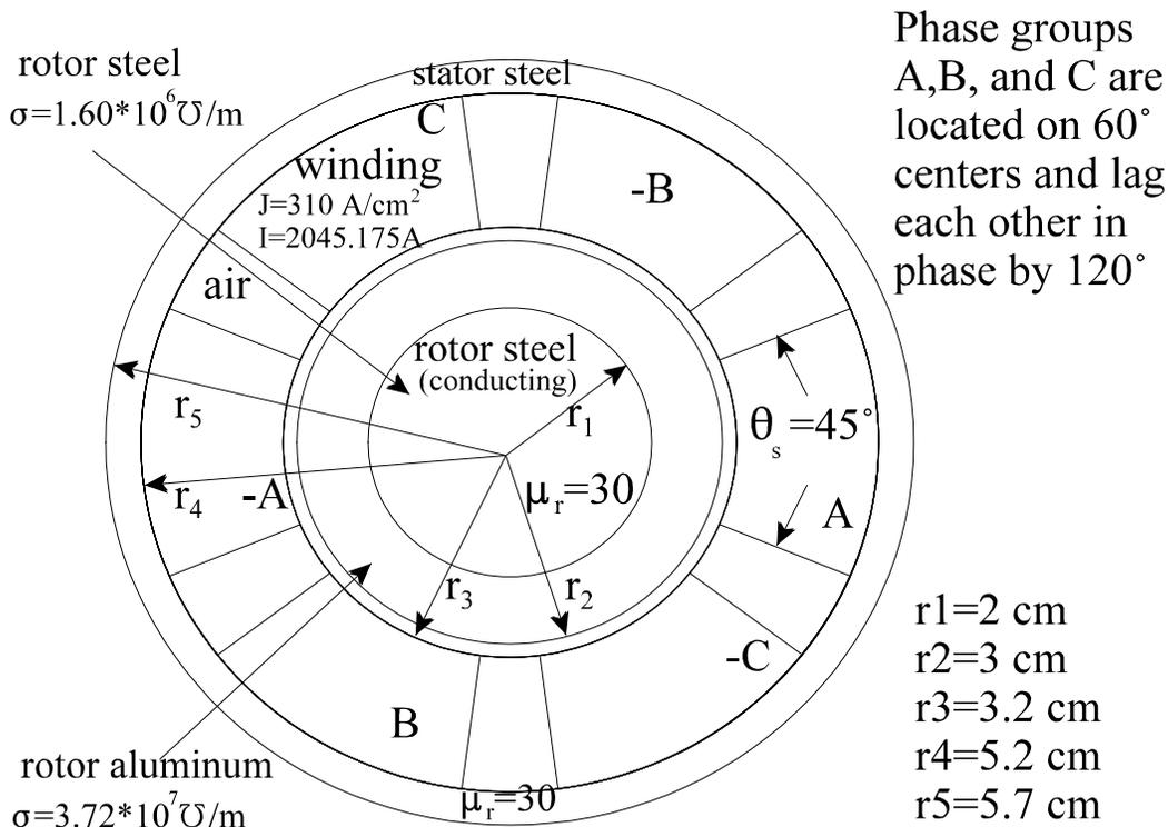
**Figure 1** Three Phase induction motor problem with a 45 degree winding spread per phase, holding  $J$  constant at 310 A/cm<sup>2</sup>.
