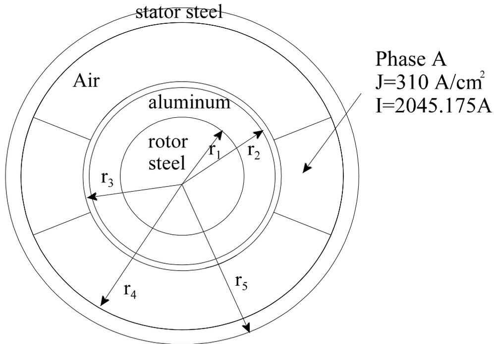
**Figure 2** Single phase induction motor problem excited at 60 Hz.
