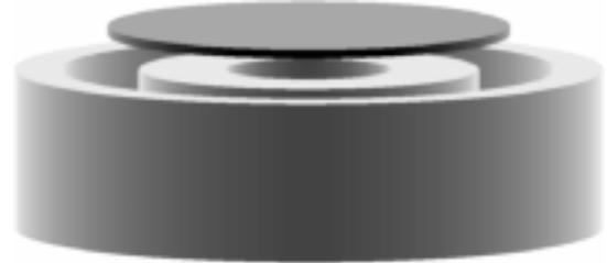
Fig. 1. TEAM Workshop problem 28: An electrodynamic levitation device
